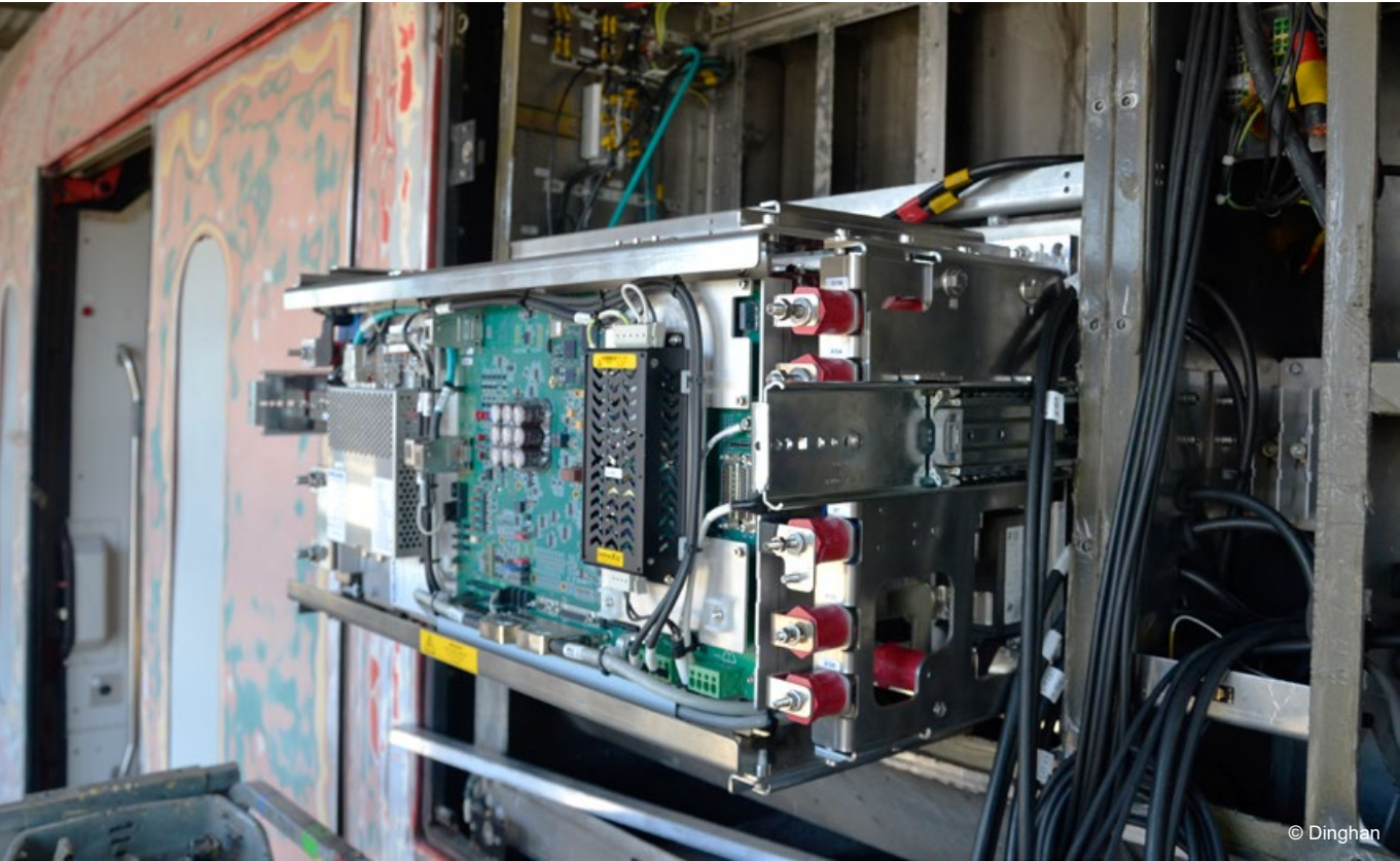
The highly efficient SMARTconverter DC had to be installed in the tightest of spaces.
